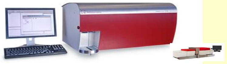
Fatty acid calibration was done once per month with reference milks produced at Cornell. The instrument tests about 50 to 70 samples per hour for all components, NPN/urea, and all fatty acid parameters. The automated model runs 600 samples per hour.
